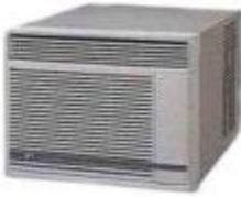
This is a self-contained air conditioning system which requires a hole to be made in an external wall or window to accommodate. These systems are used in many applications where there is no location for an external condensing unit. Air return is done via the front fascia and discharges the cooled air via a louver assembly on the front fascia also.
